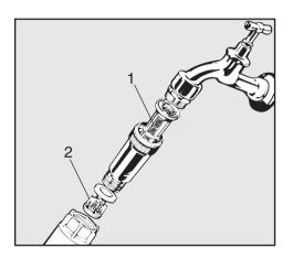
Clean the large area filter, 1, and fine filter, 2, replace with new filters, if necessary.
